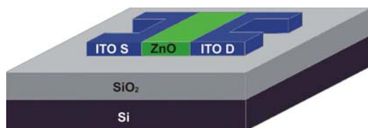
Fig. 3 Schematic of the TFT assembly used in this work
